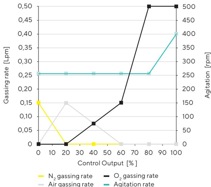
**Figure 1:** Setup of advanced pO<sub>2</sub> controller
