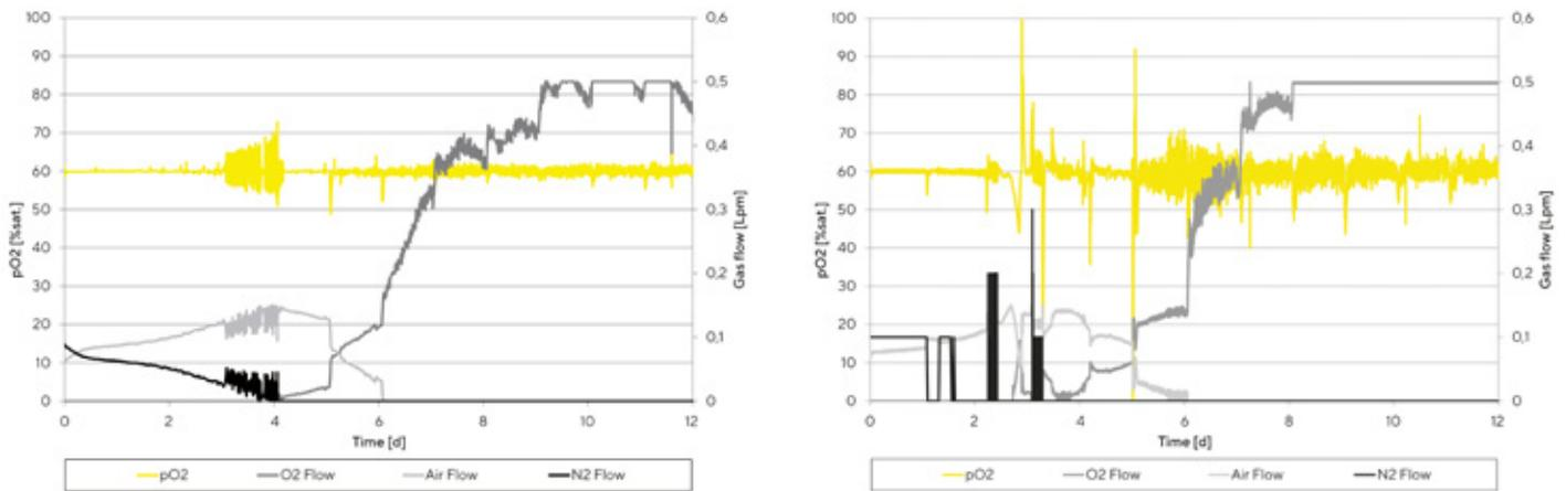
Figure 3: pO<sub>2</sub> and gassing trend – Univessel® Glass 5 L – ring sparger – Biostat® B-DCU (left) Biostat® B (right)
