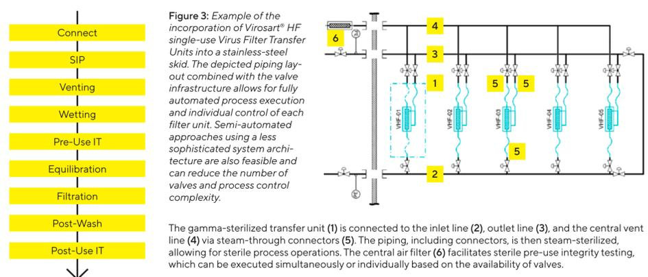
Figure 3: Example of the incorporation of Virosart® HF single-use Virus Filter Transfer Units into a stainless-steel skid. The depicted piping layout combined with the valve infrastructure allows for fully automated process execution and individual control of each filter unit. Semi-automated approaches using a less sophisticated system architecture are also feasible and can reduce the number of valves and process control complexity.
