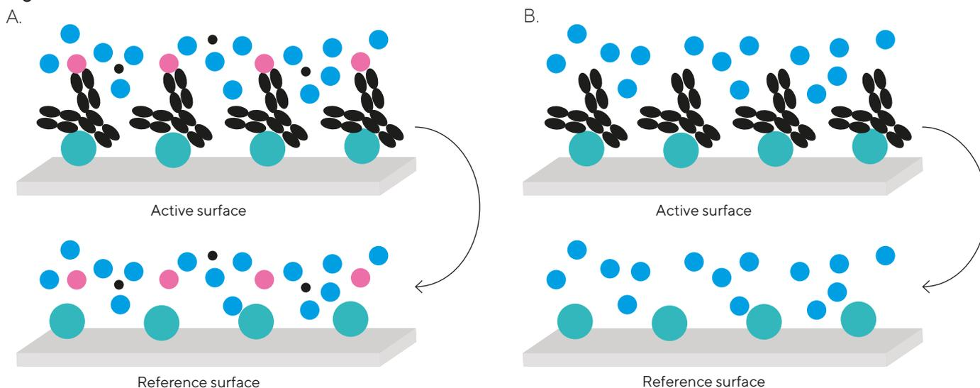
*Note.* Analyte-containing sample solution is injected across the ligand-containing active surface and a suitable reference surface (A), which allows reference subtraction of the reference surface. Buffer blank is also injected across the same active and reference surfaces (B) and the observed response is used for double reference subtraction, which helps compensate for bulk, non-specific binding and baseline drift.
