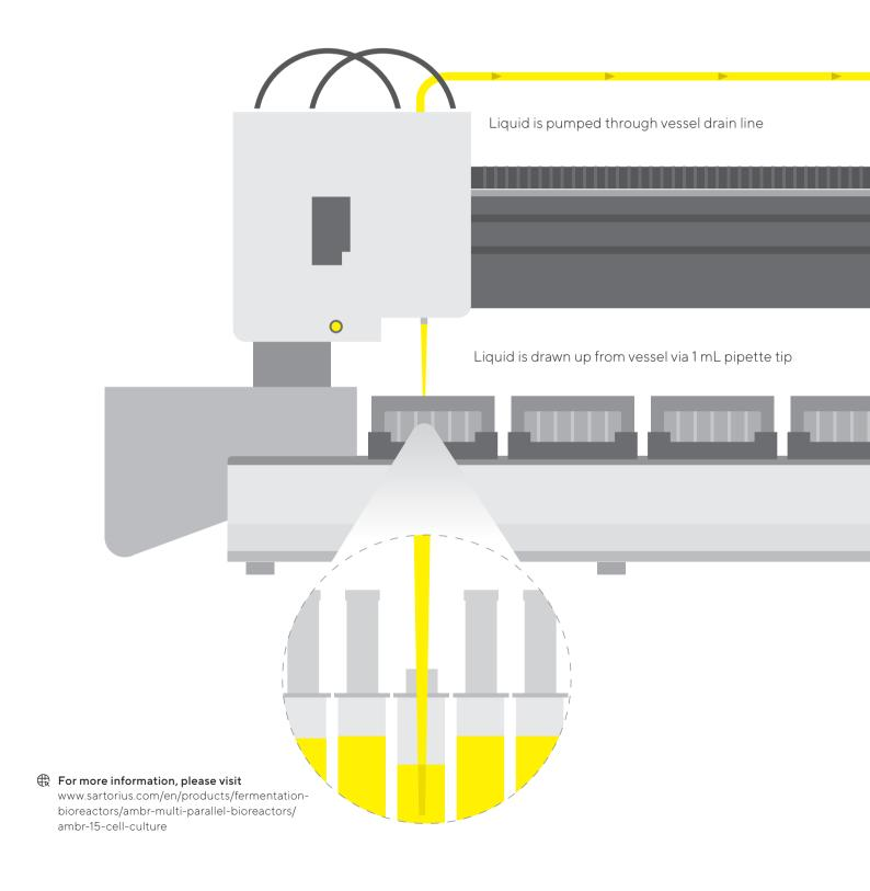
A dedicated 1 mL pipette tip mandrel collects a sterile tip and moves down to the height corresponding to the final volume required in the microbioreactor.
