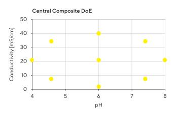
Note that the center point is repeated 5 times. This allows for the statistical significance of the experiment to be determined.
