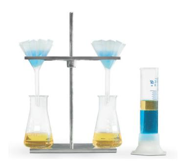
Grade 480 is impregnated with stabilized silicon, thus rendering it hydrophobic: It retains water, but allows solvents to flow through. The flow stops automatically when the entire solvent has passed through. In many applications, this phase separator paper eliminates the need to use separating funnels.
