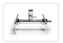
Combisart® Manifolds, 1-, 3- and 6-Branch Made of high-grade stainless steel (B.S. 304S31 | AISI 304); accommodates any type of vacuum funnel. Stainless steel three-way valves (taps) allow the vacuum for each filter holder to be individually controlled and each holder to be sterilely vented. The low height of the manifold ports is particularly advantageous for working on a clean bench.
