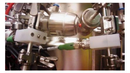
Contact temperature sensor at addition valve array
